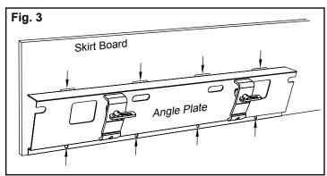
**Step 3. Weld the angle plate to the skirt board.** Stitch weld top edge with 1/4" (6mm) weld, 2" (50mm) long, in at least 4 places. Plug weld bottom edge 4 places in holes provided (Fig. 3).
